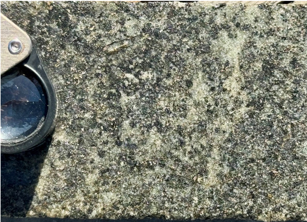
Prairie Lake Project phoscorite rock in drill core containing abundant (circa 50%) apatite (sugary, pale-green mineral)
